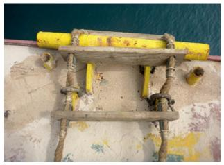
Pilot ladder incorrectly secured to the deck using D-shackles to choke the side ropes.
